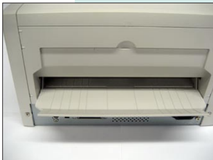
An access door on the rear of the unit, when opened, becomes an exit tray for an alternate, straight paper path for the feeding of thin, thick or smaller media.
