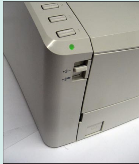
Up to three buttons on the control panel can be programmed to allow for quick, simple scanning to a pre-registered location using pre-registered settings.
